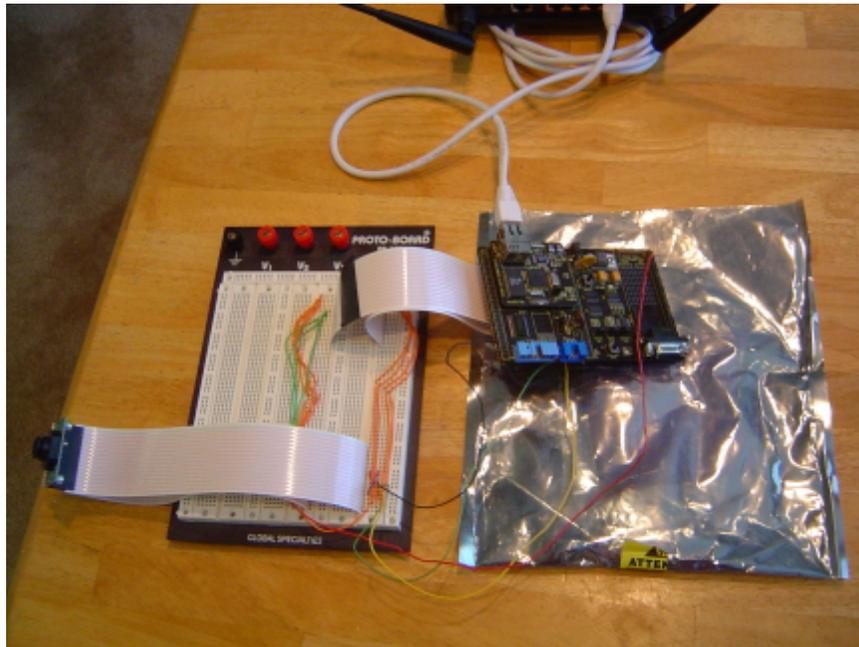
**Figure 8. EZ80F91 to breadboard wiring**
